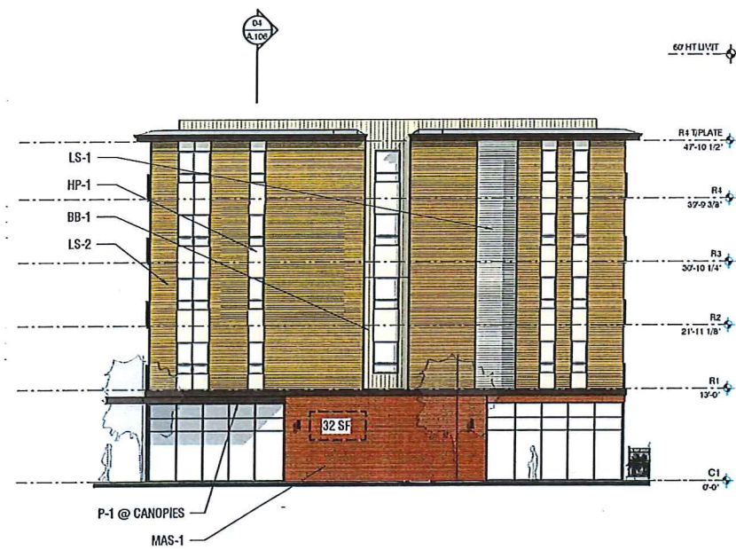
BLDG. D NORTH ELEVATION SCALE: 3/32" = 1'-0"
